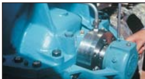
External cartridge GPAC Pump Worthington Ingersoll-Dresser Pump. liquor (Australie).
